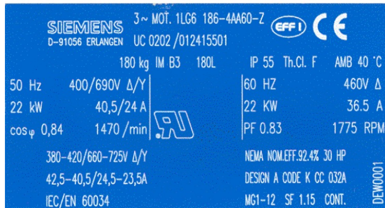
Figure 3-4: Name plate of a 22 kW motor
