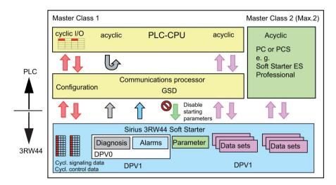
Figure 9-2 Communication principle
