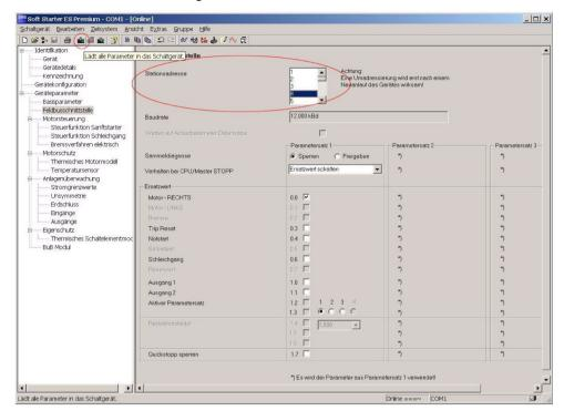
9. Select the "Load to switching device" icon in the toolbar.
