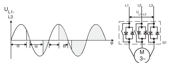
The diagram below shows the method of operation of the 3RW44 soft starter:
