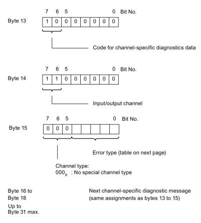
Figure 9-7 Configuration of the channel-related diagnostics
