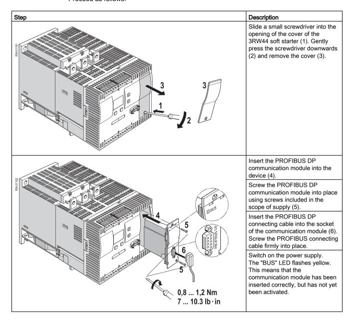
9.4 Activating the PROFIBUS DP communication module (fieldbus interface) and setting the station address
