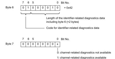
Figure 9-5 Configuration of identifier-related diagnostics
