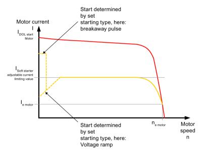
Figure 7-5 Current limiting with soft starter
