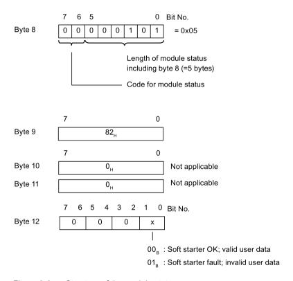
Figure 9-6 Structure of the module status
