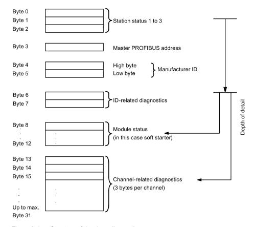
Figure 9-4 Structure of the slave diagnostics
