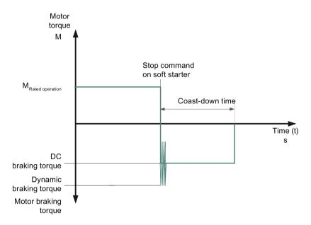
Figure 7-8 Combined braking
