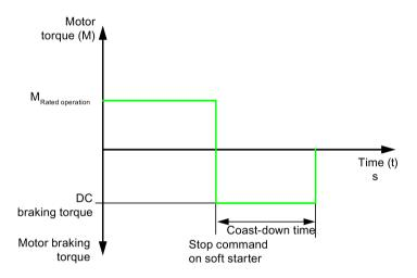
Figure 7-9 DC braking
