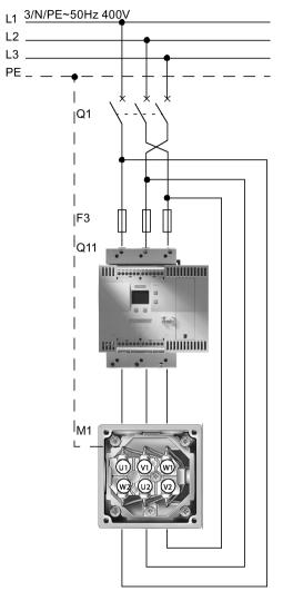
Motor rotation in line phase direction
