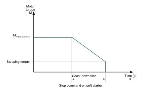
Figure 7-7 Soft stop/pump stop
