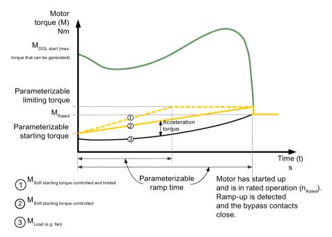
Figure 7-3 Function principle of torque control
