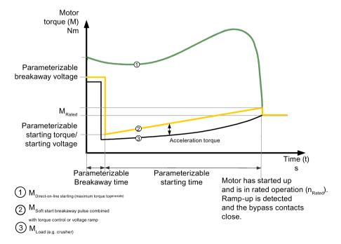
Figure 7-4 Function principle of torque control breakaway pulse
